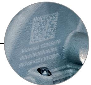
Example of a DataMatrix code
